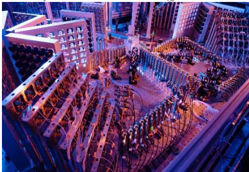
The Chinese quantum computer Jiuzhang 2.0 based on a photonic processor. Chao-Yang Lu, Chinese University of Science and Technology.
